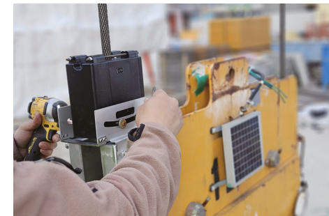
Real-time wire rope inspection
